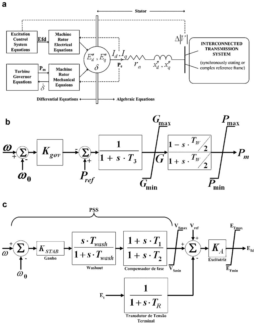
Figure 6 (a) A hydropower plant connected as SMIB system. (b) Speed Governor and Hydraulic Turbine Model. (c) Fast Static Exciter and Power System Stabilizer Model.
