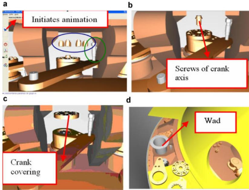
**Figure 4** (a) Beginning of maintenance animation of superior trunnion plugs. (b) Removing the screw of crank axis. (c) Removal of the crank covering. (d) Removal of wad. [Color figure can be viewed in the online issue, which is available at [www.interscience.wiley.com](http://www.interscience.wiley.com).]
