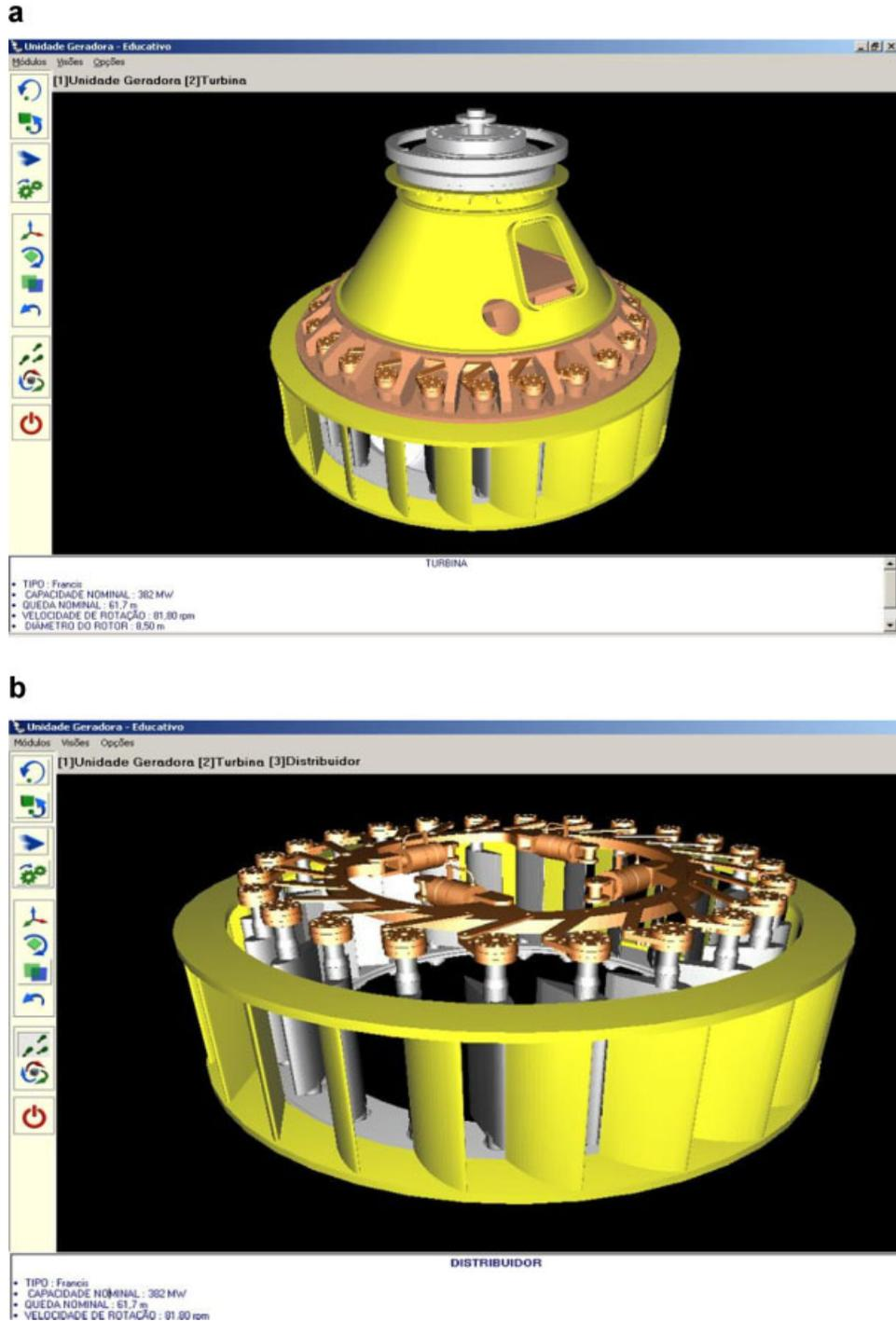
**Figure 3** (a) Turbine selected by picking over VGU. (b) Turbine Distributor System selected in level internal. [Color figure can be viewed in the online issue, which is available at [www.interscience.wiley.com](http://www.interscience.wiley.com).]
